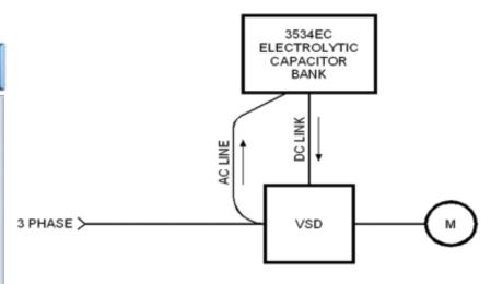
2.5KW & BELOW, 0 - 0.5 SECOND, 100% OUTAGE PROTECTION USING ELECTROLYTIC CAP RESERVOIR SINGLE CABINET POWERED FROM AC LINE
