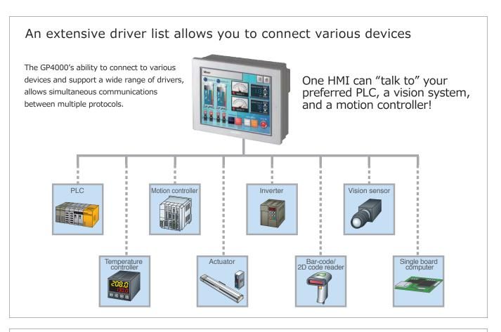
Screen data can be updated by using the data transfer tool, even without a software license.
