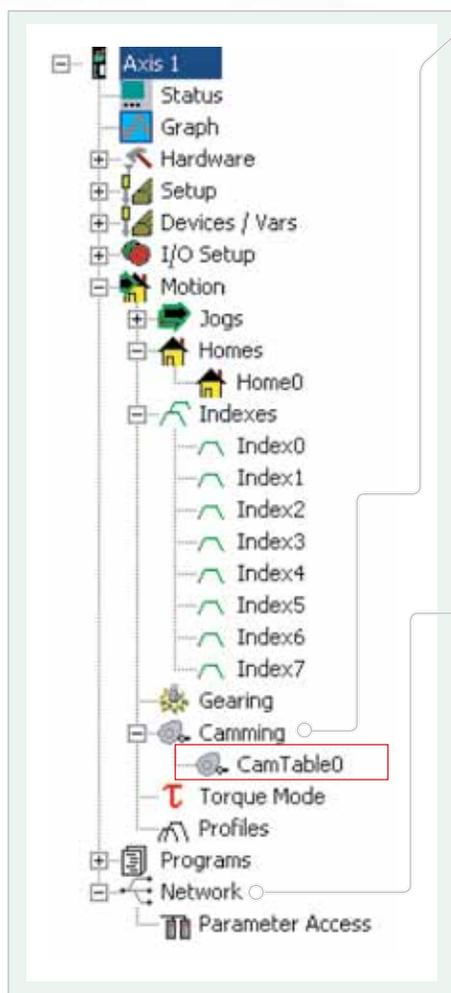
**Camming** – Cams make set-up and programming of complex motion profiles easy. The use of real-time programs provides smooth transitions when switching between cam profiles on-the-fly. Cam data is easily imported within PowerTools Pro and the cam graphing tool features multiple interpolation types.
