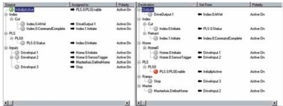
• **Indexes** – Indexes are set up easily by filling in the screen’s blanks to create an index profile. Select from incremental, absolute, registration, or rotary plus and minus types. Choose the time base of the index by selecting either real-time or synchronized to a master. Over 100 user-defined indexes are available with the Epsilon EP.
