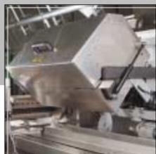
Longitudinal sealing unit with fold-down mechanism
