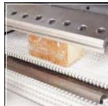
Motorized belt in the transversal sealing and cutting unit
