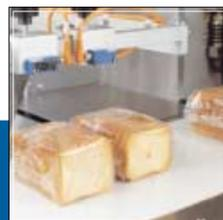
Device for the detection and rejection of empty and double packs
