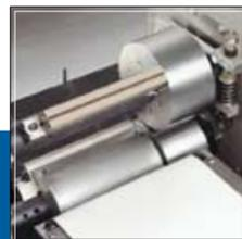
Transversal sealing and cutting unit
