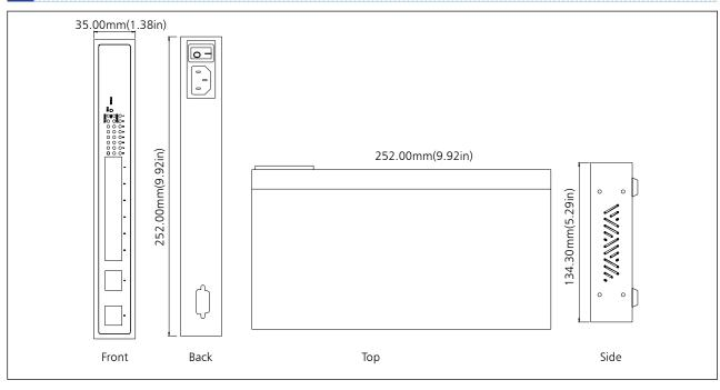
16-port 10/100Base-TX and 1-port 100Base-FX Web-Smart Ethernet Switches
