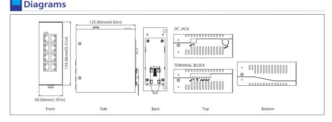
5-port 10/100Base Fast Ethernet Industrial Unmanaged Ethernet Switches
